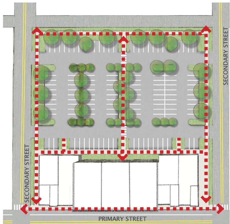
FIGURE 30.2 Pedestrian Sidewalk Network
