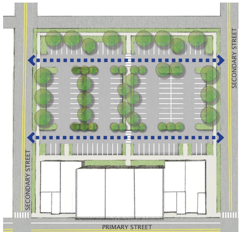
FIGURE 30.3 Vehicular Cross Access
