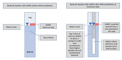
As shown above, LNAPL collecting above bedrock cannot enter the well since the part of the well open to the formation is too deep. Well data from wells with logs and water level data included in the RIWP is presented below:
